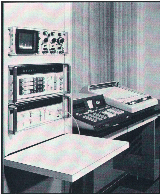
Fig. 3. The Model 3571A Tracking Spectrum Analyzer also functions under programmable calculator control through the HP Interface Bus, giving an automatic measurement and data-reducing system that shortens test time and decreases the possibility of measurement error. A packaged calculator-based system that includes the analyzer is known as the Model 3045A Automatic Spectrum Analyzer.
