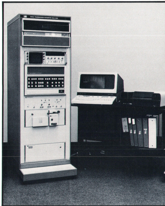
Fig. 1 Model 5453A Transmission Parameter Analyzer is both a general-purpose stimulus-response test instrument and a special-purpose analyzer for performance tests on voiceband data channels and components. Table I lists some of its capabilities.
